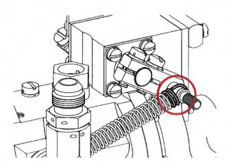
10. Reinstall the adjusting rod , secure with self-locking nuts.
