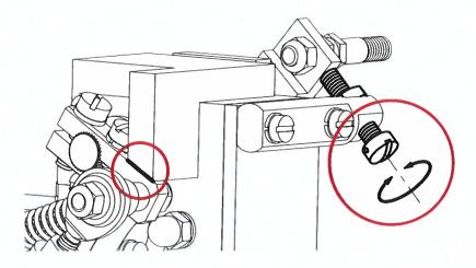
If the angular difference is big enough to turn the end stop more than 4 turns, reposition the lever feedback lever on its shaft by one tooth.
