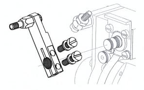
c) Install new BC lever with the new pin in the same position (or very close) and fix with original screws and washers.
