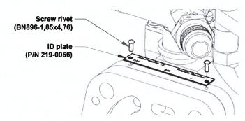
a) Using a small slotted screwdriver and suitable nose pliers, carefully release and remove the ID plate from the governor.
