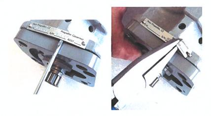
b) Using suitable nose pliers, carefully turn the screw rivets counterclockwise to remove them from the governor.
