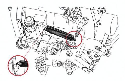
c) Hook up the new spring at one end to the holder. Do NOT slide the other end of the spring onto the pin. Do not reinstall the adjusting rod now!
