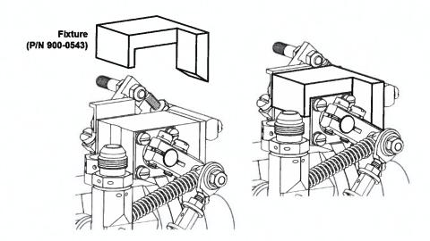
b) The feedback linkage lever (P/N 220-0023-3-1) must match with angular surface of the fixture – see the picture. To adjust angle of the lever, use end stop of the BC lever.
