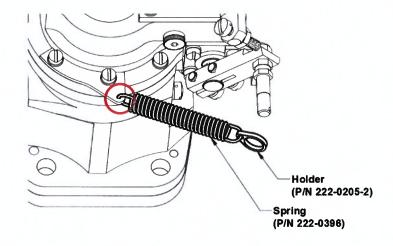
d) Install the spring on the BC lever pin.
