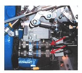
Disconnect pitch lock solenoid connector and beta switch connector from engine harness.
