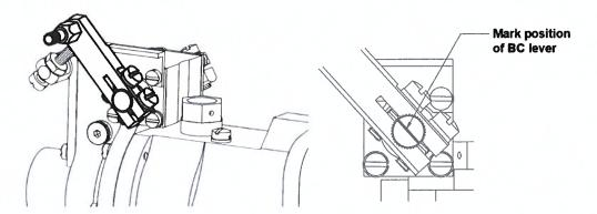
b) Remove the safety wire from BC lever fixing screws. Release the screws and remove the BC lever from the shaft. Original BC lever is marked 220-0023-5-1.
