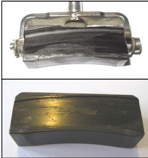
FIGURE 1: Excessive wearing of the carbon block
